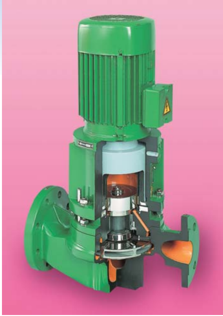
Inline-volute casing pump type KMV with hermetically sealed magnetic coupling. Capacity up to 60 m 3 /h (300 USgpm), differential head up to 60 mLC (300 ft).
