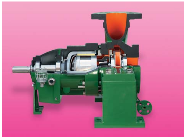
Volute casing pump type PRM acc. to API 685 with hermetically sealed magnetic coupling, centerline mounted.
