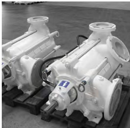
Intermediate flange at stage casing
