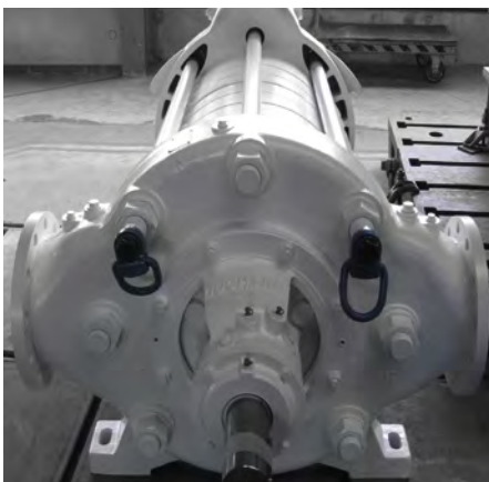
Two flanges in one suction casing
