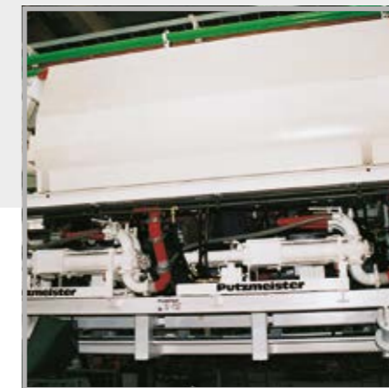
Left: A KOV 1050 pumps the injection mortar behind the ring segment Right: Space-saving installation with two KOV 550 Duo underneath a 6 m 3 agitating trough
