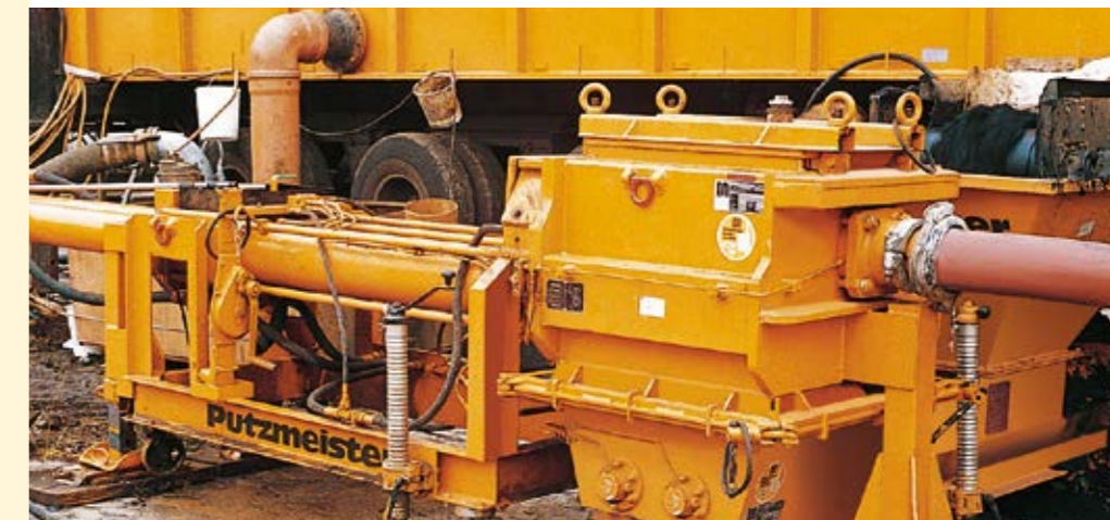
Mobile dewatering and pumping station
