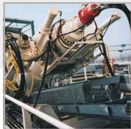
Auger conveyor with two muck pumps of type KOS 1480 (Botlek tunnel, Netherlands)
